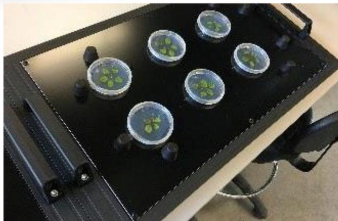
**Suitable for a range of sample types,** the high-resolution sensors on the HyperAixpert enable rapid digital analysis of phenotyping traits thereby delivering optimised results for experiments in genetics, plant research and breeding, plant cultivation products as well as detecting plant stress and diseases.
